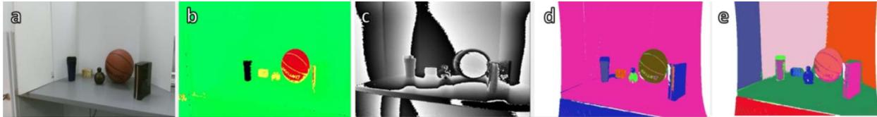
Figure 3. a, b, and c) The captured scene Kinect color frame in *RGB*, in *Lab*, and depth frame, respectively. d) The 3D clustered point cloud using  $k=8$  clusters and detecting 9 objects. e) The 3D clustered point cloud using  $k=10$  clusters and detecting 11 objects.
